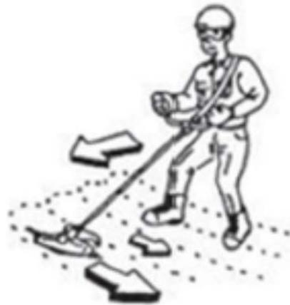
5.3.4. Keep cutting deck parallel with the ground. Do not tilt the nylon cutting or blade head during operation.
