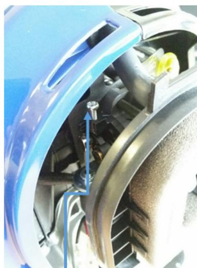
Idle speed adjusting screw – with air filter cover removed
