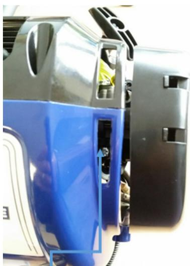
Idle speed adjusting screw
