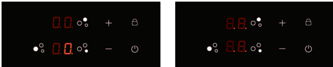
Fig. 8.: Selected cookset 0 for all the heaters. Heater selection finished
