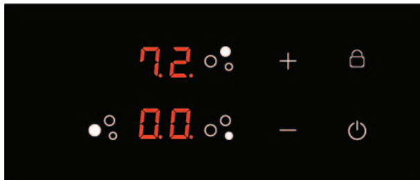
Fig. 16.: Displays showing CookTop ECO Power Limit
