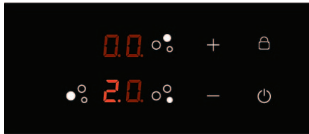
Fig. 21.: Selecting a power level for a heater
