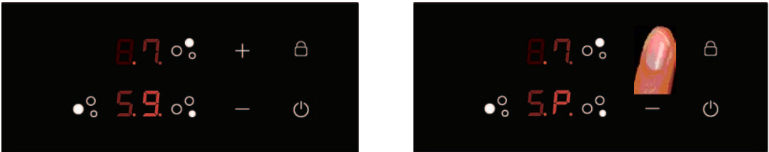
Fig. 11.: Selecting a power level with [+] [-] keys
