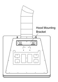
5. Carefully place the decorative chimney bottom into the recessed area of the hood body top. Secure the decorative chimney bottom to the wall using (2) ST 2.9 x 14mm mounting screws and dry wall anchors.
