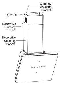
7. Fix the range hood with screws (2) ST4.2\*30mm and dry wall anchors from inside of body.
