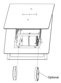
4. Install grease filter after charcoal filter is installed.
