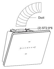
4. Align the hood body with the hood mounting bracket. Gently lower the hood until it securely engages the bracket.
