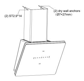
6. Carefully slide the decorative chimney top down inside the decorative chimney bottom. Raise the decorative chimney top until its holes align with holes in the chimney mounting bracket (located on the wall). Secure the chimney with 2 screws M4\*6mm.
